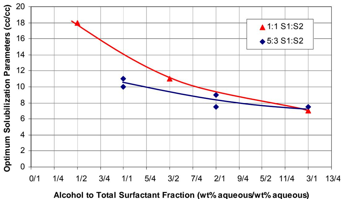
**Figure 4.** Effect of co-Solvent (SBA) concentration on optimum solubilization parameter at 1% total surfactant concentration and two ratios of Petrostep S1 to Petrostep S2.
