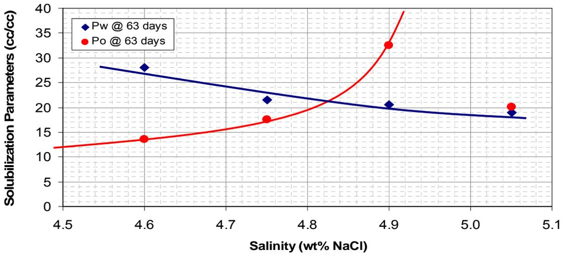
**Figure 8.** Salinity scan for samples containing 0.25 wt% Petrostep S1, 0.25 wt% Petrostep S2 and 0.125 wt% SBA at 46.1 Celsius - Trembley Oil.
