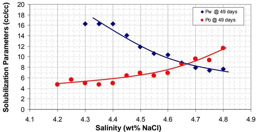
**Figure 2.** Solubilization parameters for salinity scan for a formulation containing 0.625 wt% Petrostep S1, 0.375 wt% Petrostep S2 and 2 wt% SBA with Trembley crude oil @ 46.1 Celsius after equilibrating for 49 days.
