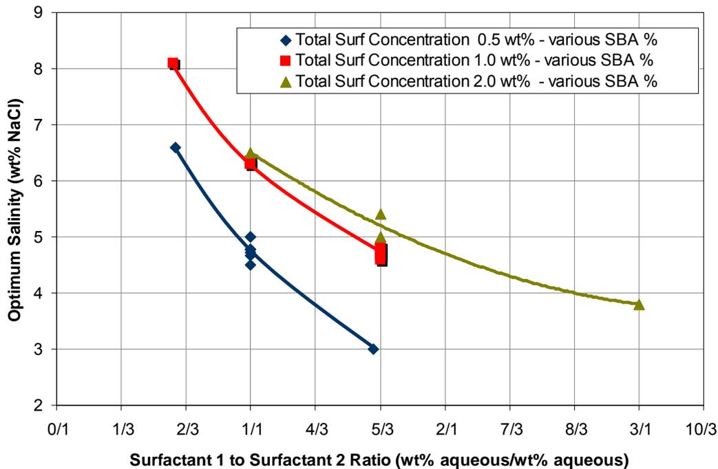
**Figure 3.** Effect of varying Petrostep S1 to Petrostep S2 ratio on optimum salinity with various SBA concentrations. Oil is Trembley crude oil @ 46.1 Celsius.
