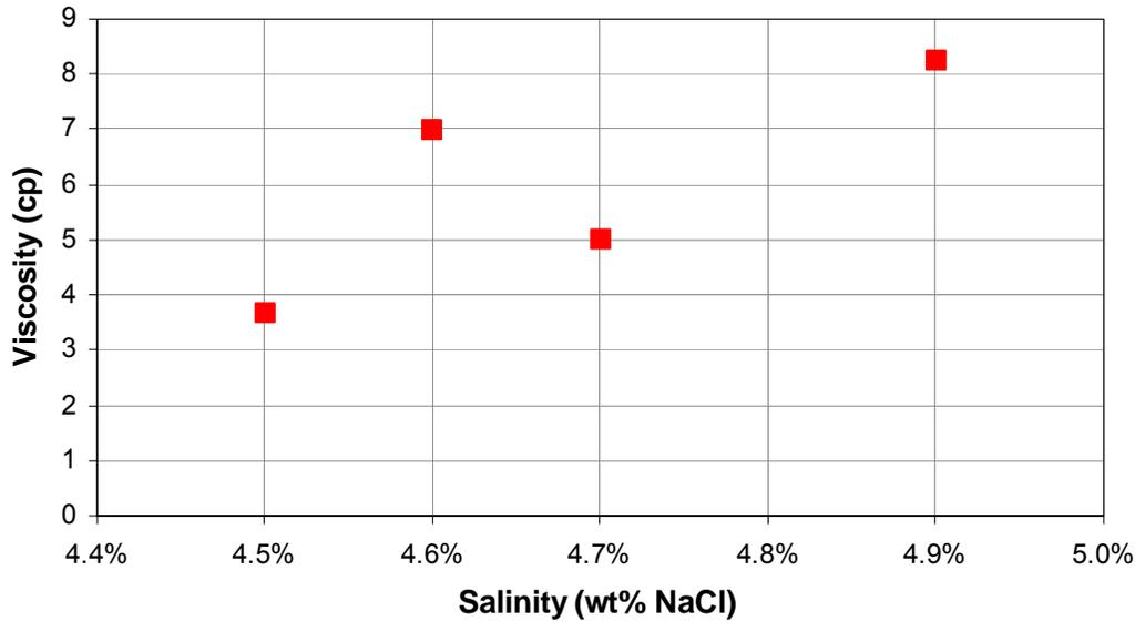
**Figure 9.** Viscosities of type III microemulsion close to optimum salinity for samples containing 0.25 wt% Petrostep S1, 0.25 wt% Petrostep S2 and 0.25 wt% SBA at 46.1 Celsius with Trembley Oil. Measurements conducted at a shear rate of  $75 \text{ s}^{-1}$ .
