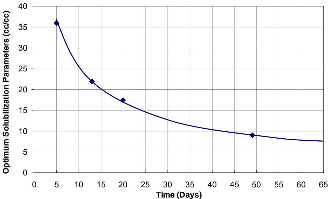
**Figure 6.** Optimum solubilization parameters plotted against time to estimate equilibration time for salinity scans containing 0.625 wt% Petrostep S1, 0.375 wt% Petrostep S2 and 2.0 wt% SBA at 46.1 Celsius with Trembley crude oil.
