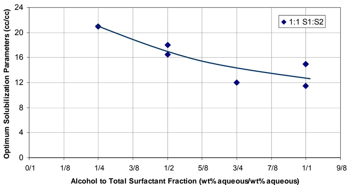
**Figure 5.** Effect of co-solvent (SBA) concentration on optimum solubilization parameter at 0.5% total surfactant concentration and different alcohol:surfactant ratios.
