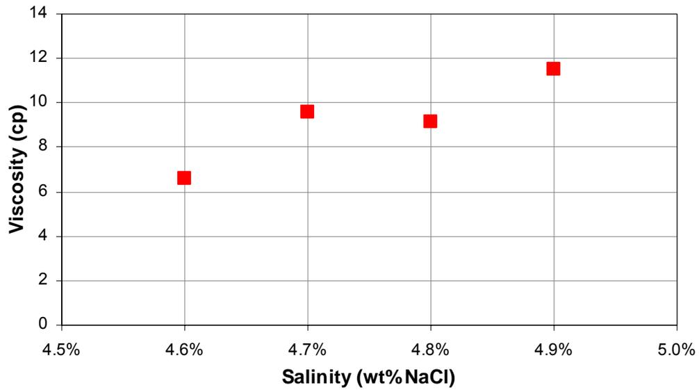
**Figure 7.** Viscosities of microemulsion phase close to optimum salinity for samples containing 0.25 wt% Petrostep S1, 0.25 wt% Petrostep S2 and 0.125 wt% SBA at 46.1 Celsius- Trembley Oil. Measurements conducted at a shear rate of  $75 \text{ s}^{-1}$ .
