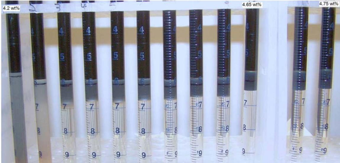
**Figure 1.** Photo of a salinity scan for a formulation containing 0.625 wt% Petrostep S1, 0.375 wt% Petrostep S2 and 2 wt% SBA with Trembley crude oil @ 46.1 Celsius after equilibrating for 49 days. Salinity from 4.2 to 4.75 wt% NaCl (left to right) at increments of 0.05 wt% NaCl.
